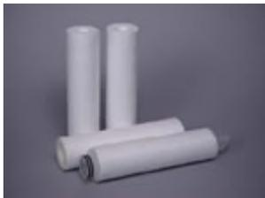
GDMB Melt blown cartridges are manufactured by a continuous spun bonding technology that assures a consistent product. 100% all polypropylene construction gives wide chemical compatibility and extremely low extractables. These cartridges offer exceptional value in both removal efficiency and dirt holding capacity where protection of more expensive membrane filters is important.
